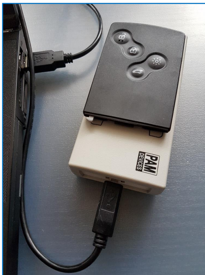
Fig. 1 Transponder programmer Master Key III
