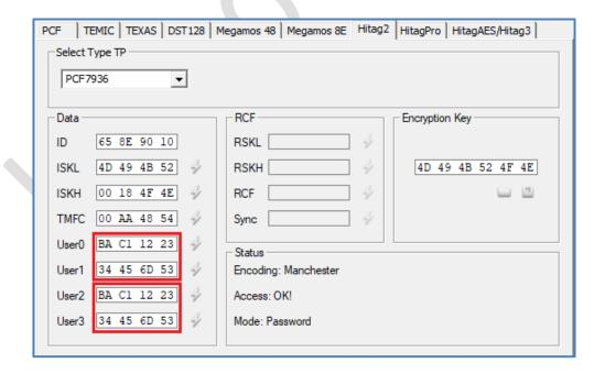
**NOTE:** Fail to read data from transponder may mean that your HITAG2 programmer does not support **fast initialization**. Repeat steps 1 to 5 using different HITAG2 programmer.
