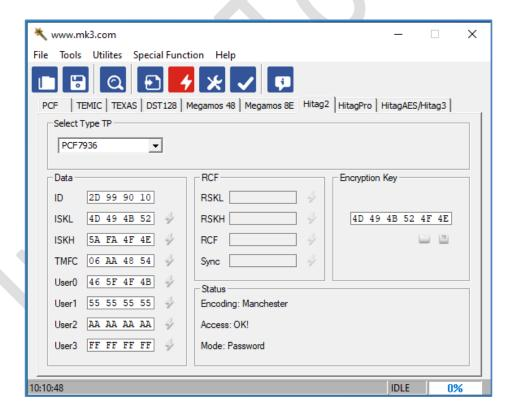
6) For example, you need to make a key with value BA C1 12 23 34 46 7F D2. Fill fields User0 and User2 with BA C1 12 23 Fill fields User1 and User3 with 34 46 7F D2 Make sure User0 = User2 and User1 = User3! Make sure the first two bytes of User0 and User2 are equal to BA C1!
