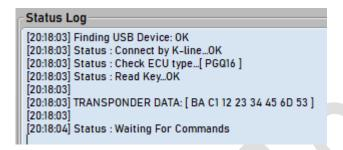
**NOTE 1**: Only key of the new type, based on **PCF7936** or on **T5**, set to **Biphase** encoding, can be read here.
