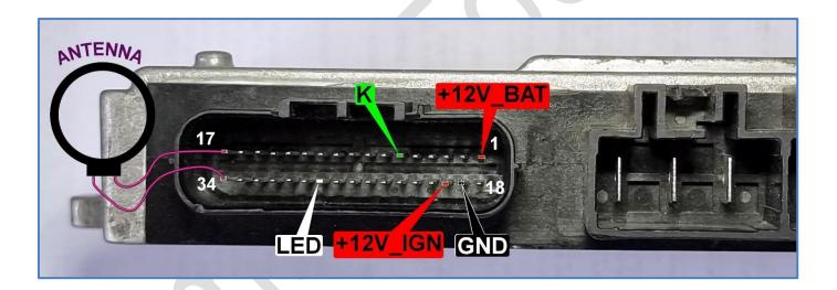
Antenna and LED are optional components. They should be connected only to test key validity on-the bench.
