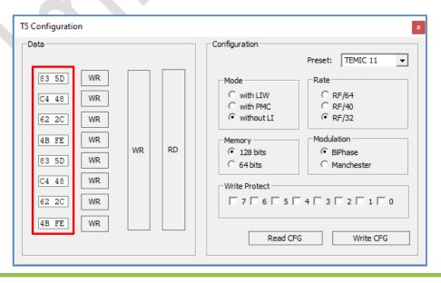
4) Write all pages and configuration to **T5**. From this point your **T5**, configured in such way, will be recognized by universal transponder programmer as **T5-11**.
