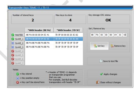
Write value of any active (marked with green) key to transponder **T5** as **TEMIC-11** using any suitable transponder programmer. Choose data with header "**BE FA**" or "**7D 5F**" depending on type of your transponder programmer.
