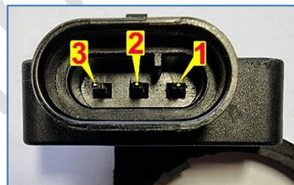
Transponder Reader (Antenna) pinout
