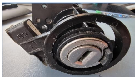
Antenna on the ignition lock
